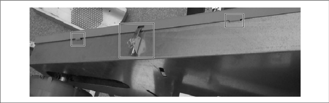
Figure 6-8 Latches for the belt guard cover
