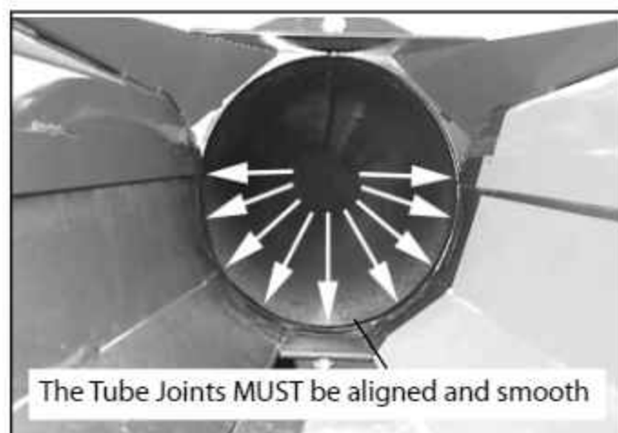
FIG. 3-71. Tube Joint Detail
