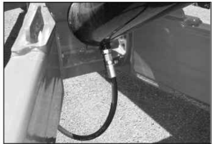
FIG. 3-47. Hydraulic Hose to the Cylinder
