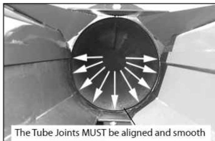
FIG. 3-5. Tube Joint Detail
