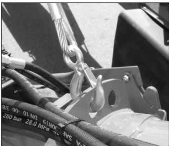
FIG. 4-4. Connecting the Lift Cable
