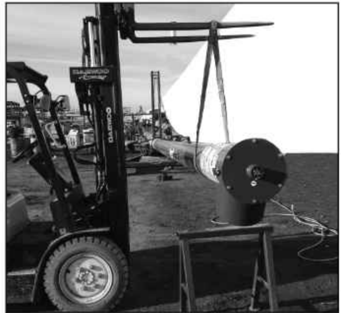
FIG. 3-32. Lifting the Discharge End of the Tube
