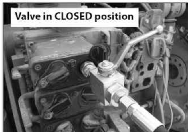
FIG. 4-5. Hydraulic Lift Shut-off Valve
