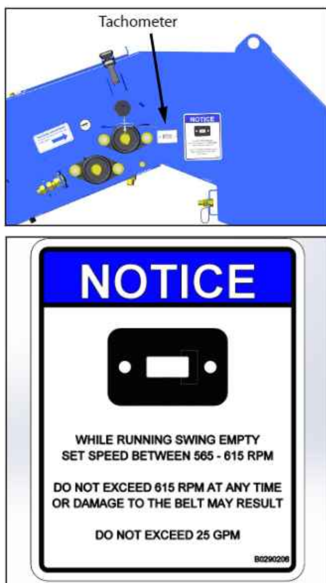
FIG. 4-7. Swing Conveyor Drive Roller Speed
