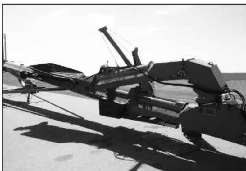
FIG. 4-10. Swing Conveyor In Transport Position
