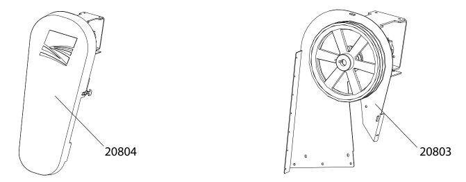
Figure 5. Safety Decal Locations for PTO-SD Option
