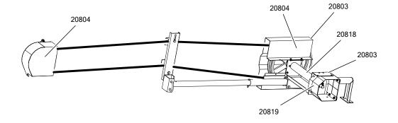
Figure 7. Safety Decal Locations for Hydraulic Drive Option
