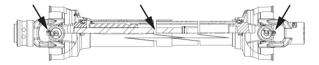
Figure 12. Typical PTO Driveline Grease Points (European)
