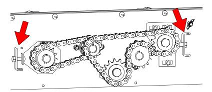
5. Tighten the chain tension roller idler bolt to 120ft-lb using a torque wrench.
