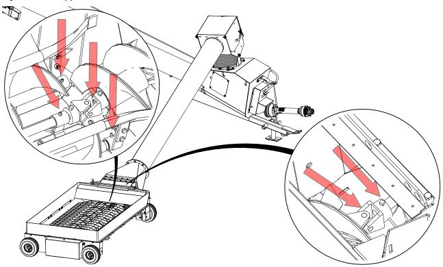
Figure 26. Upper Flighting Bearing Grease Point
