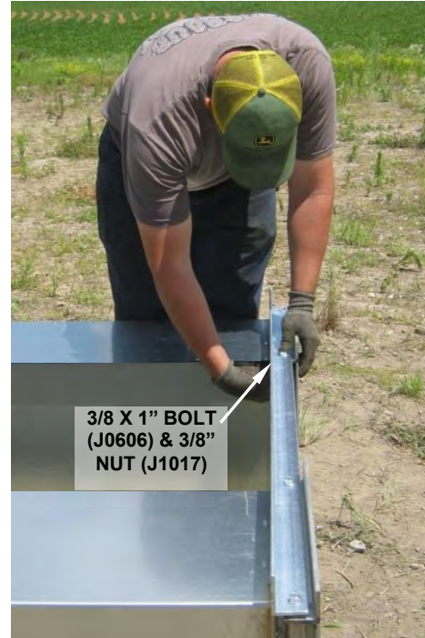
Image 2 – Bolting tie angle to flanges
