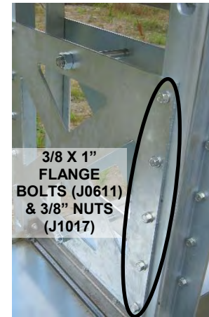
Images 7-10 – Attaching tie angles, squaring plates & alignment pins
